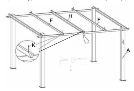
8. To attach the canopy (P) to the pergola, feed a pair of canopy poles (1 x I & 1 x J) through the canopy runners on the underside of the end pieces (G). One canopy pole should be fed through per side. Next feed the poles into the wallets sewn into the canopy (P) as show in the diagram below. Push the canopy poles together through the canopy runner on the underside of the centre roof bar (H). Repeat this step for the remaining canopy poles (4 x I & 4 x J) to hang the canopy from the frame.
