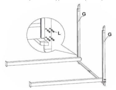
6. Attach the remaining corner posts (1 x B and 1 x A) and side piece (1 x D&E) to construct the full frame. Secure using the medium screws (16 x L with supplied washer).
