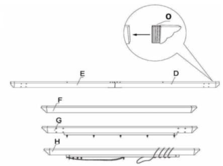
4. Build one side of the frame from two corner posts (1 x B and 1 x C) and a side piece D&E. The side piece (D&E) should be secured to the lower set of holes at the top of each post. The posts should be positioned so that the higher set of holes face outwards from the frame. Secure using the medium screws (8 x L with supplied washer).
