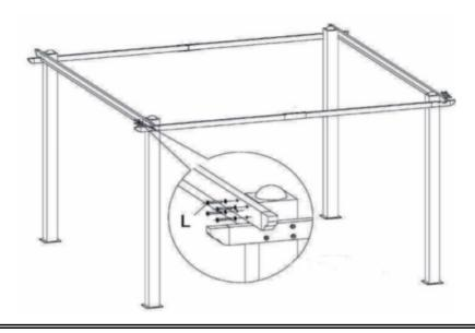
7. Attach the roof bars (2 x F, 1 x H) to the frame using the long screws (6 x K with supplied washer). The centre roof bar should be positioned so that the pull cord emerges on the opposite side of the frame to the captive canopy runners on the underside of the end pieces (G).
