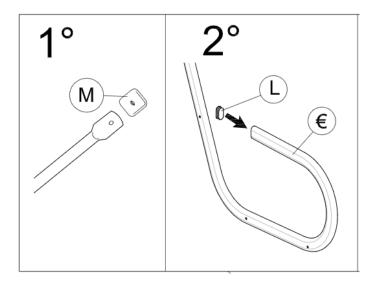
10) Attach each of the arm rests (€) to the seat and back rest frames of the seat (\$) &(#) using the screws advised in the diagram below. Use the springs (O) to attach the swing seat arms to the top of the canopy frame.
