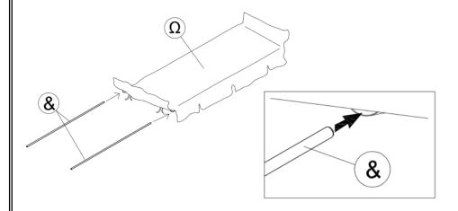
6) Attach both rounded ends of the canopy frame (%) onto the straight canopy bars (&) ensuring that you slot the pole of (%) into the grooves of the plastic fixtures (K) on each side of the canopy frame.
